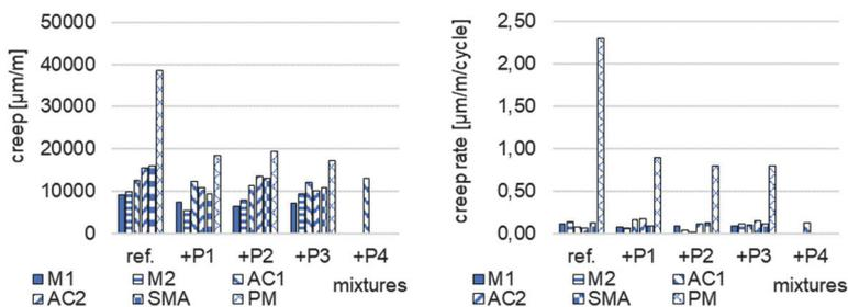
Figure 2 cyclic compression tests: creep (left) and creep rate (right)
