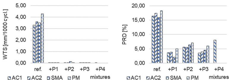
Figure 3 Wheel tracking tests: WTS (left) and PRD (right)
