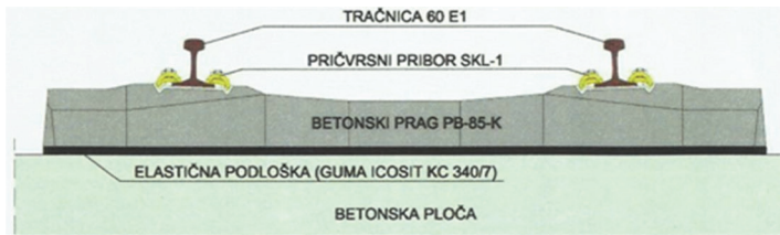
Figure 9 Vibration measurement on a concrete base with an elastic bedding [1]
