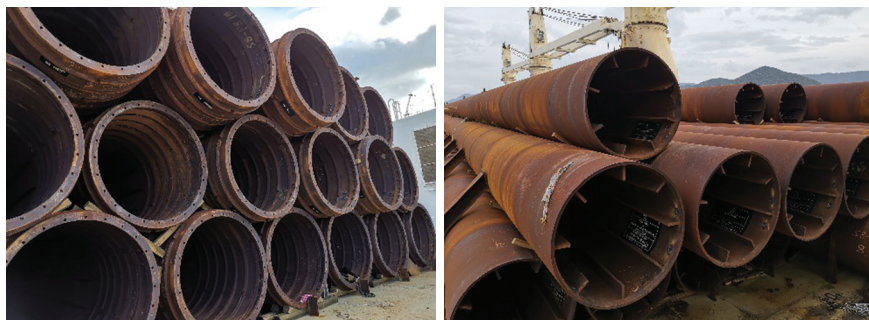
Figure 1 Shear rings of pile head and pile shoes with stiffening pile shoes
