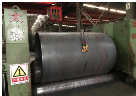
Figure 2 Standard segment rolling and forming
