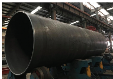
Figure 3 Fit-up of standard segments
