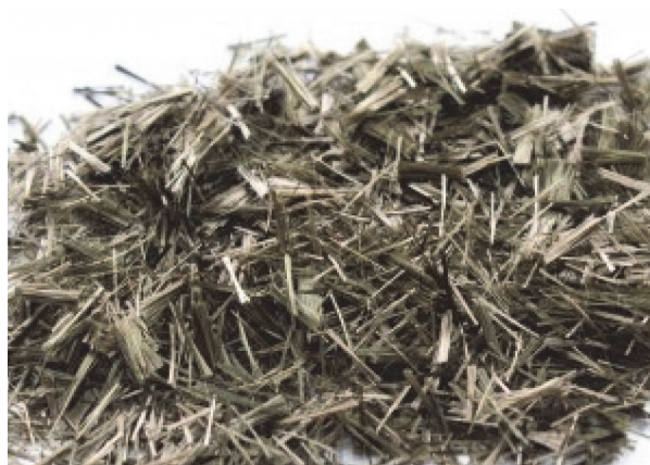
Figure 1 Basalt fiber, the fiber length is 20-25 mm and the diameter is 13-20 mm
