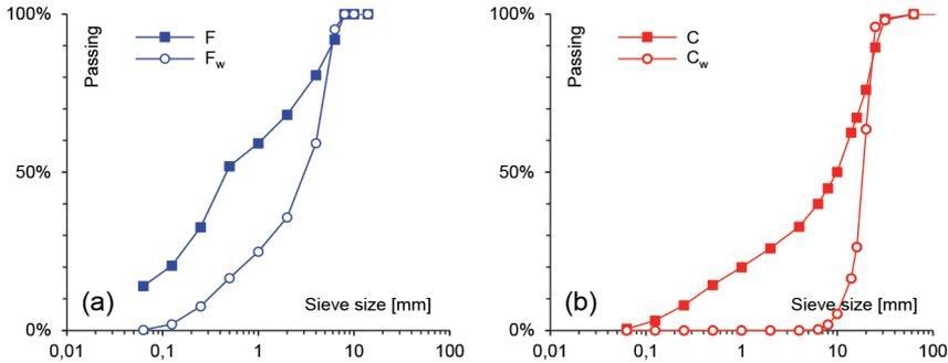
Figure 2 Gradations of selected stockpiles: a) fine aggregates F and  $F_w$ , b) coarse aggregates C and  $C_w$
