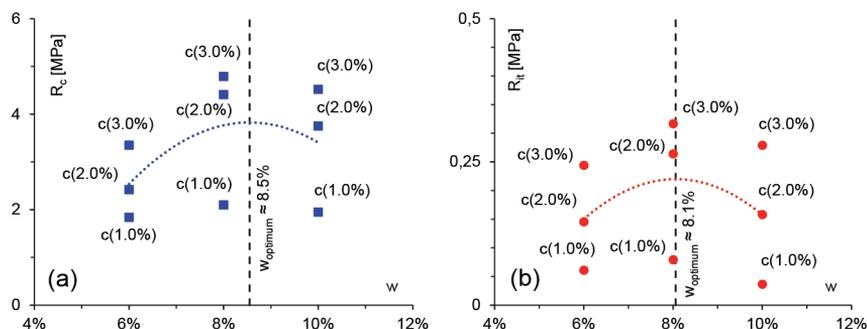
**Figure 4** Mix design of FF<sub>w</sub>CC<sub>w</sub> mixture: R<sub>c</sub> (a) and R<sub>t</sub> (b) vs. c and w
