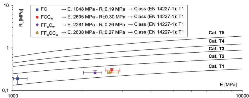
**Figure 5** Figure 5. E and Rt experimental results and classification (EN 14227-1)
