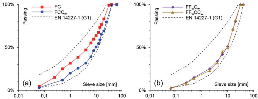
Figure 3 Final gradations of mixtures: a) FC,  $FCC_w$ , b)  $FF_wC_w$ ,  $FF_wCC_w$
