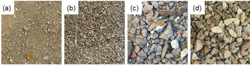
Figure 1 Images of the selected CDW aggregates: a) F, b)  $F_w$ , c) C, d)  $C_w$
