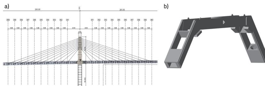
Figure 6 Layout of stay cables: a) Layout of stay cables, b) Link anchor box on pylons
