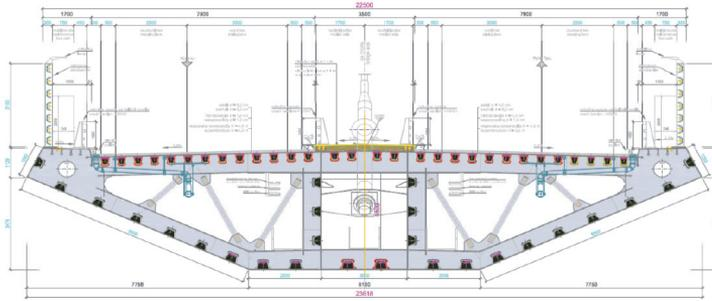
Figure 7 Standard cross section with stay cables
