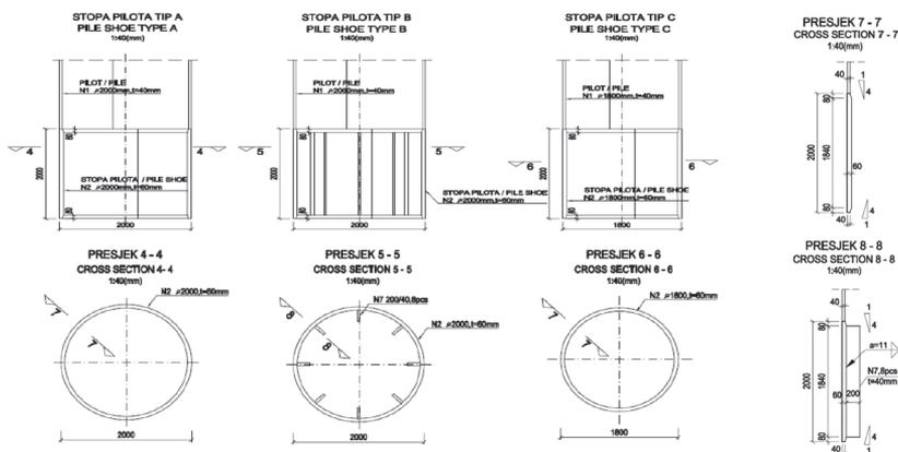
Figure 3 Details of pile toes
