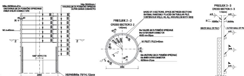
**Figure 2** Details of pile head
