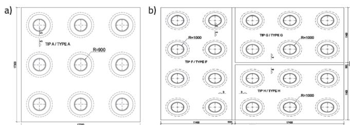
Figure 4 Configuration and joint detail of concrete bottom slab
