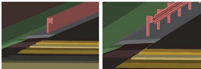
**Figure 2** The difference between traffic barrier for lower levels (LOD200) and implementation specifications (LOD400)
