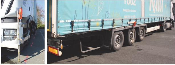
**Figure 2** Water tanks at front most prominent point and inner endpoint of the test vehicle
