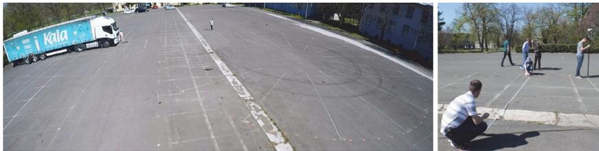
**Figure 5** Test drive and measurements of test vehicle's swept path widths
