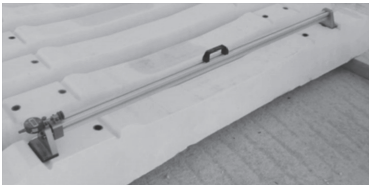
Figure 3 Measuring the shoulder width with a gauge within 0.01 mm. [6]
