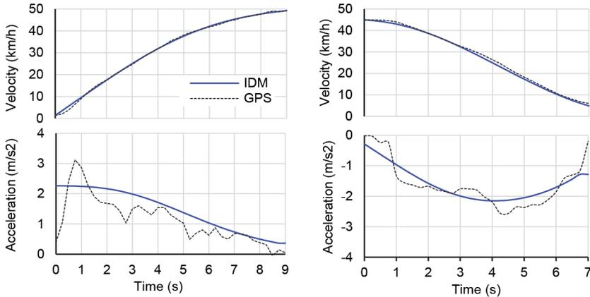
Figure 3 Field vs predicted cinematic profiles for the acceleration and deceleration manoeuvres
