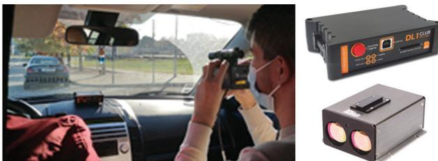
Figure 1 Data acquisition system: Left – measuring the gap to the leading vehicle; top right – datalogger; top bottom: LIDAR
