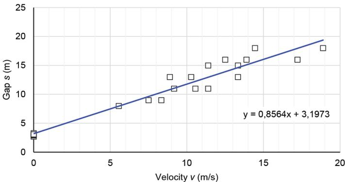
Figure 4 Linear regression of s-v data points in steady-state conditions
