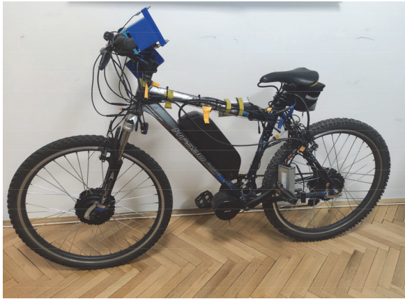
Figure 4 Electric bicycle with all kits and test equipment installed
