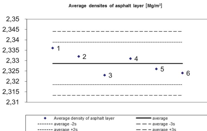
**Figure 2** Average densities and standard deviations of asphalt layer determined from 30 measurements of all 6 participating laboratories
