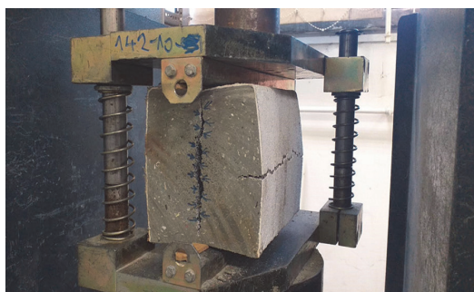
Figure 4 Cracking of recycled plastic beam in splitting test
