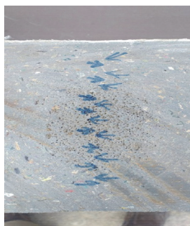
Figure 5 The resealed crack in the beam made of recycled plastic after the load is released
