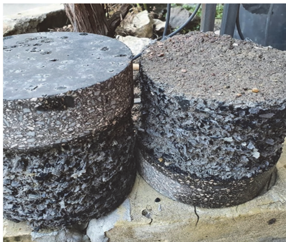
Figure 7 Core samples of trial sidewalk with bonded layers
