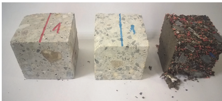
Figure 1 The three samples tested (from left. samples with gravel, crushed stones and plastic aggregate)
