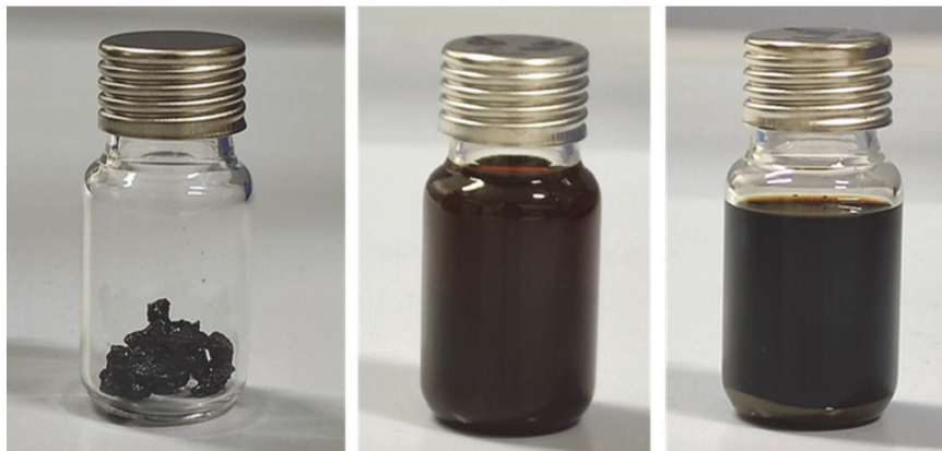
Figure 1 RAP sample: unsolved (left), solved in toluene (middle) and separation of binder and aggregate matter after centrifuge (right)
