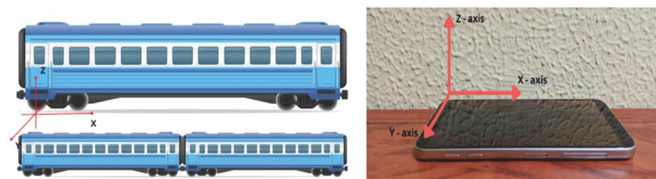
Figure 3 Direction of measurements taken by the mobile phone in relation to train movements
