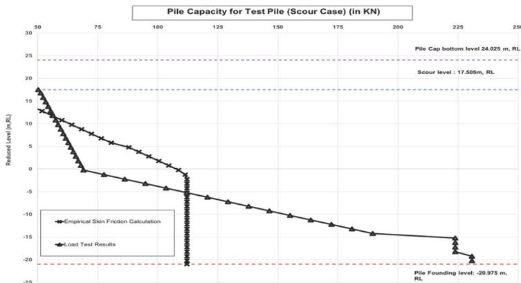
Figure 6 Skin Friction Comparison based on theoretical and load test results
