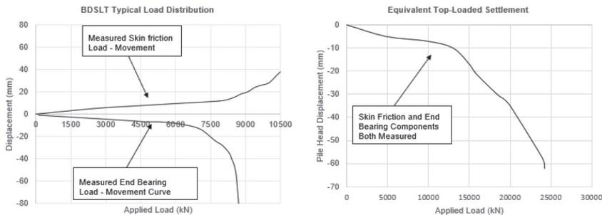
Figure 3 Conversion of BDSLT curve to conventional top-loaded pile load test result
