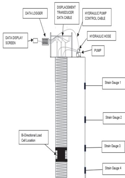
**Figure 5** Load Cell Positioning provided in the pile
