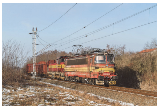
Figure 1 Electric loco class 230 together with diesel loco class 731 pulling a short freight train
