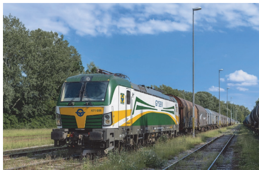
Figure 2 Siemens Vectron AC, equipped with last-mile module (diesel engine), with freight train outside of the electrified track
