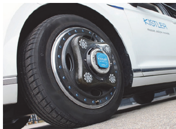
Figure 1 Dynamometrical wheel (source: kistler.com)
