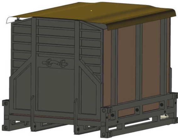
Figure 6 View of the platform-container with side walls and unfolded roof
