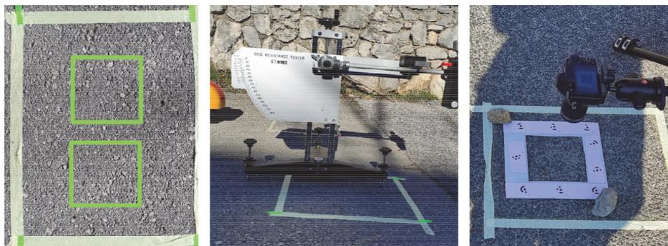
**Figure 1** An example of analysed pavement section measured with SRT and photographed by orthographic photogrammetry method
