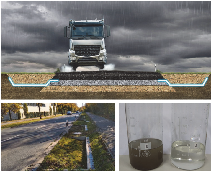
Figure 2 Generic design of a filter trench (top), test fields (bottom left) and unfiltered vs. filtered runoff from test fields (bottom right)
