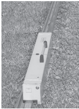
Figure 2 RAILPROF 1000 handheld device (on the left) and rail roughness graphs for locations with different exploitation periods (on the right) in the wavelength domain [4]
